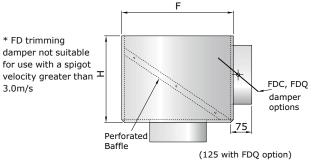
\* Please note the total installed height assumes an overlap of 30mm on the diffuser neck / plenum connection.
