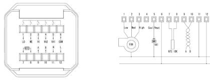
LCF Touch Modbus – Manual mode wiring diagram for 2-pipe fan coil
