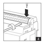
Installation with Z179 cascade plug accessory (not included in the scope of delivery)
