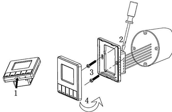
Insert the screw driver in the plastic teeth of thermostat. Clockwise rotation of the screwdriver will separate front cover from base plate. Please follow the wiring diagram to connect the wires. Fix the thermostat base plate to the wall through the four screw holes with distance between axes of 60 mm. Fasten base plate and front cover. Do not press the panel in order to protect LCD.
