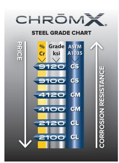
**ChrōmX 9000** (formerly MMFX<sub>2</sub>® concrete reinforcing steels) can be specified as **ASTM A1035 CS** either Grade 100 or 120. This chromium steel provides high corrosion protection for severe convive environments caused by seawater, aggressive soils and deicing salts. Designers can meet 100-year service life requirements called for on many infrastructure projects by specifying ChrōmX 9000.
