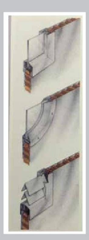
As standard, all door and frame components are supplied in a single pack etch primer - stoved.
